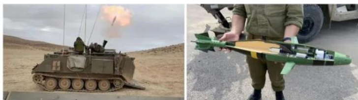
Left image: 120mm CARDOM/ Iron Sting mortar system onboard an IDF M1064 Armoured Personal Carrier in 2022. Source: IDF
