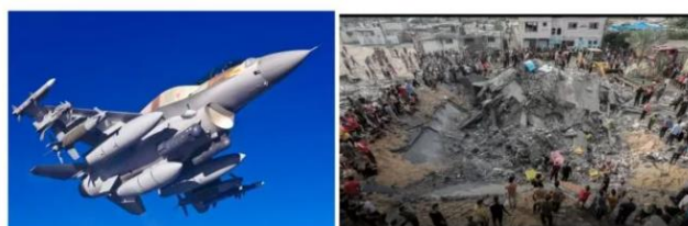
Left image: SPICE 2000 mounted on the middle pylons of this F-16I aircraft. Source: Rafael
